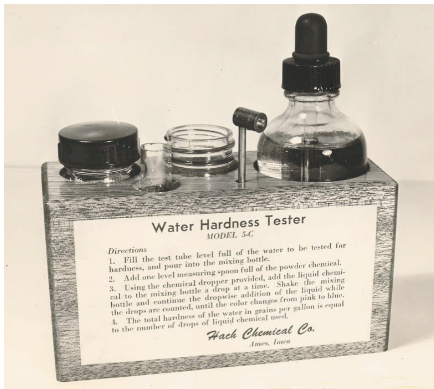
Model 5-C Water Hardness Tester, mahogany block, 1952.
